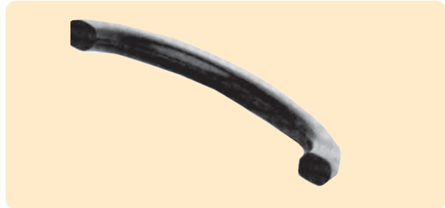
Figure 10-1: Characteristic compression set — high deformation—seen as flattening on all contact surfaces.
