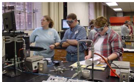
Faculty and student visitors make CdSe nanoparticle solutions (left) and perform UV-vis spectroscopic analysis on them (right).
